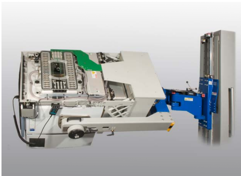
Figure 5. J750 combined with X750 system.
