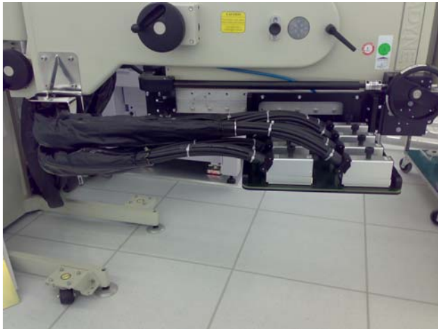
Figure 3. IDPS cable connection to the PIB.
