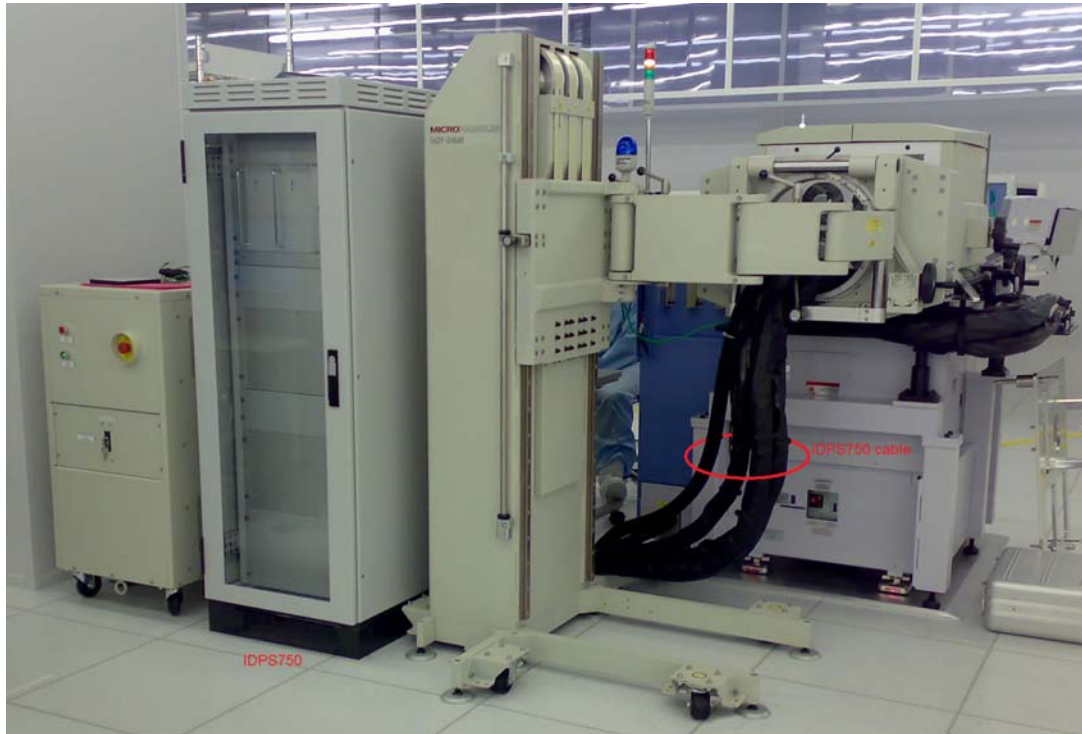
Figure 2. J750 Test Cell with IDPS 750.
